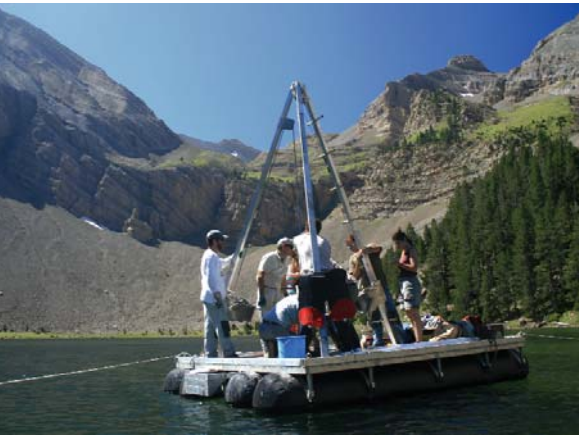
Fig. 4. Drilling sediment cores from lake deposits in one of the high mountain lakes in Sobrarbe Geopark, Spain. The cores record environmental and climatic changes at high altitudes
