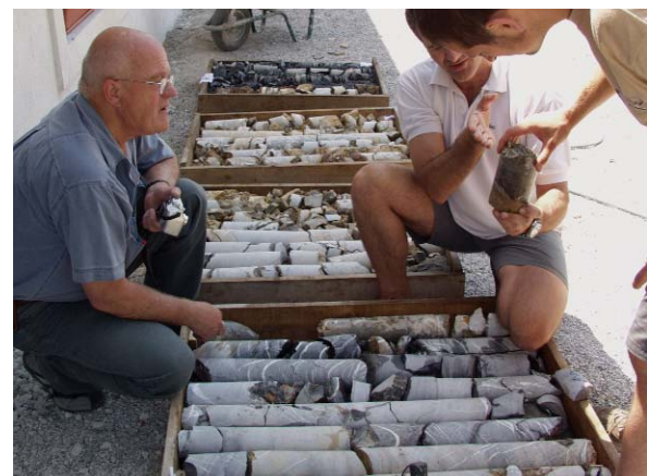
Fig. 3. Scientists from the Croatian Geological Survey analyse core samples of dolomite and limestone rocks in order to discover the nature of a subsurface sequences of rock layers
