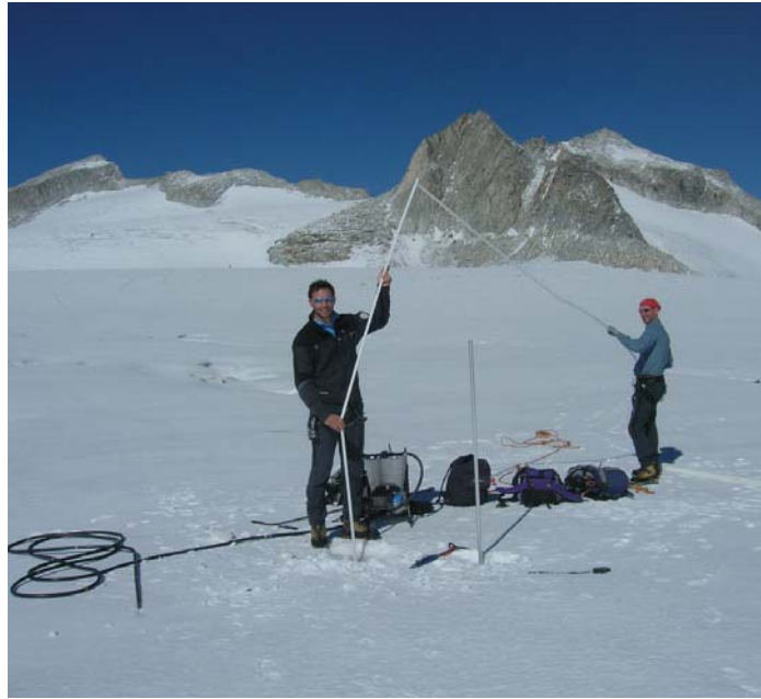
Fig. 9. Recording measurements for mass balance studies of the Adamello Glacier, Adamello - Brenta Nature Park, Italy
