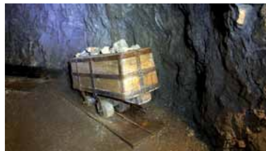
A tram used for transporting copper ore in the Sunnpau Show Mine.
